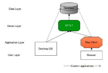
Users can edit data with a Desktop GIS application or with an internet browser through a web application. Data is then submitted to a WFS-T service that pass edits to the Data Layer. Outside OGC standards, data can be edited from a Desktop GIS application that directly save edits in a server DBMS. Also, web applications can offer the possibility to edit data using custom systems.
