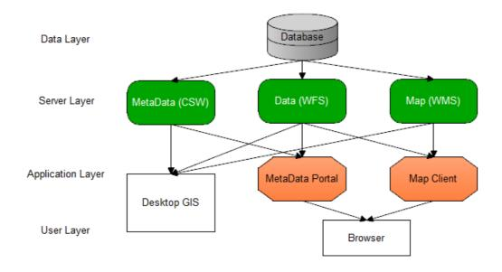
The Data Layer stores data: this operation can be handled with a Spatial enabled DBMS (like PostgreSQL or MySQL), with files (like ESRI Shapefiles, XML or JSON files) or using a WFS service.
